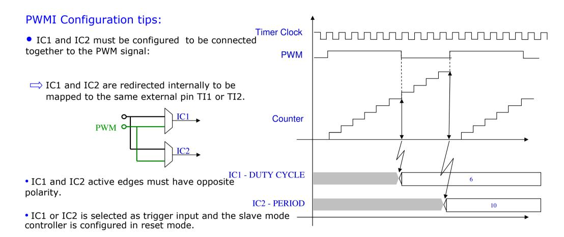
The PWM Input functionality enables the measurement of the period and the pulse width of an external waveform.
