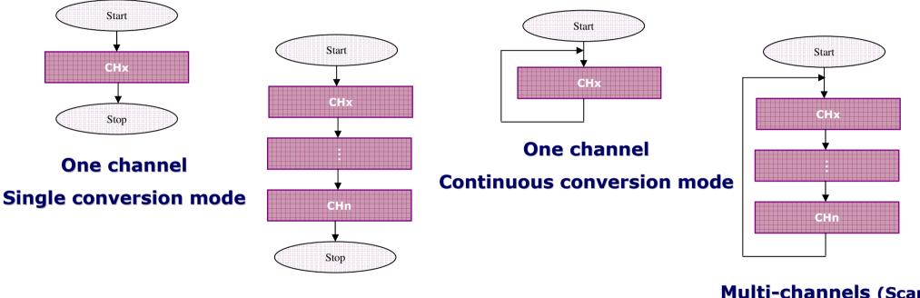
Multi-channels (Scan) Single conversion mode Multi-channels (Scan) Continuous conversion mode
