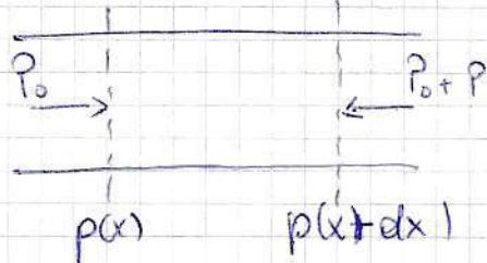
$$\frac{dF = S(p(x) - p(x + \Delta x))}{-S \frac{\partial p}{\partial x}} = \rho S dx \frac{\partial^2 \xi}{\partial x^2}$$
