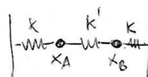
$$\left\{ \begin{array}{l} M\ddot{x}_A + Kx_A + k'(x_A - x_B) = 0 \\ m\ddot{x}_B + Kx_B + k'(x_B - x_A) = 0 \end{array} \right.$$
